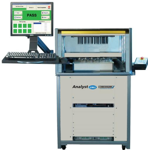
The MultiWriter ISP System is appropriate for circuit boards and multi-board panel assemblies requiring on-board code programming and verification of serial bus ISP devices. MultiWriter is available only as an integrated element of a CheckSum-developed application package that includes a bed-of-nails fixture and associated test program operating on an Analyst in-circuit test system.
