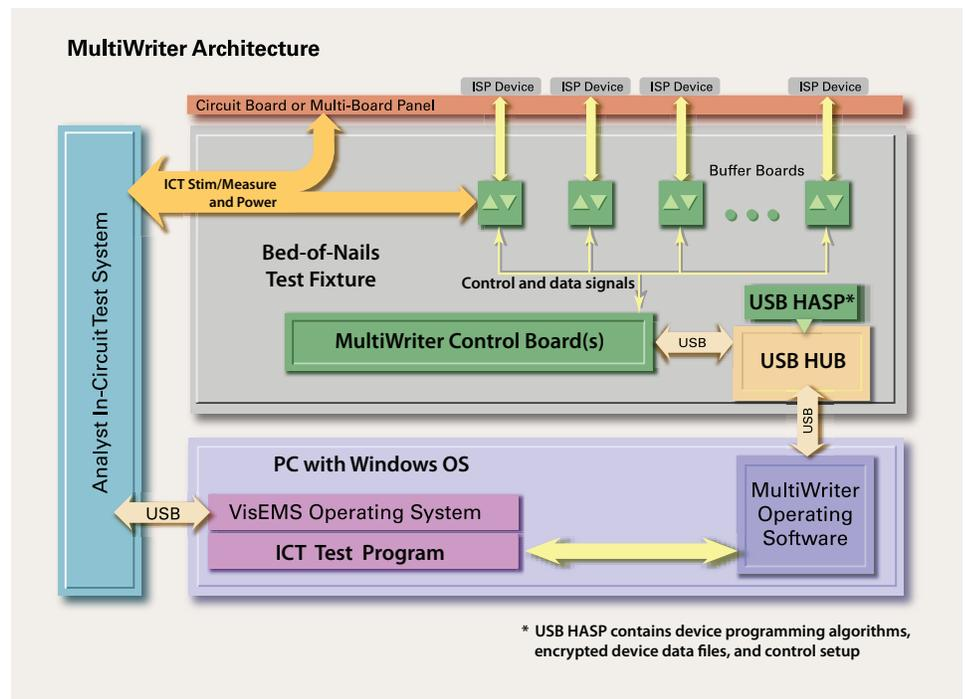
*Installing the ISP Control Module and one or more buffer modules inside the test fixture adds complete ISP programming capability to the Analyst in-circuit tester. No expensive tester-based hardware is required.*
