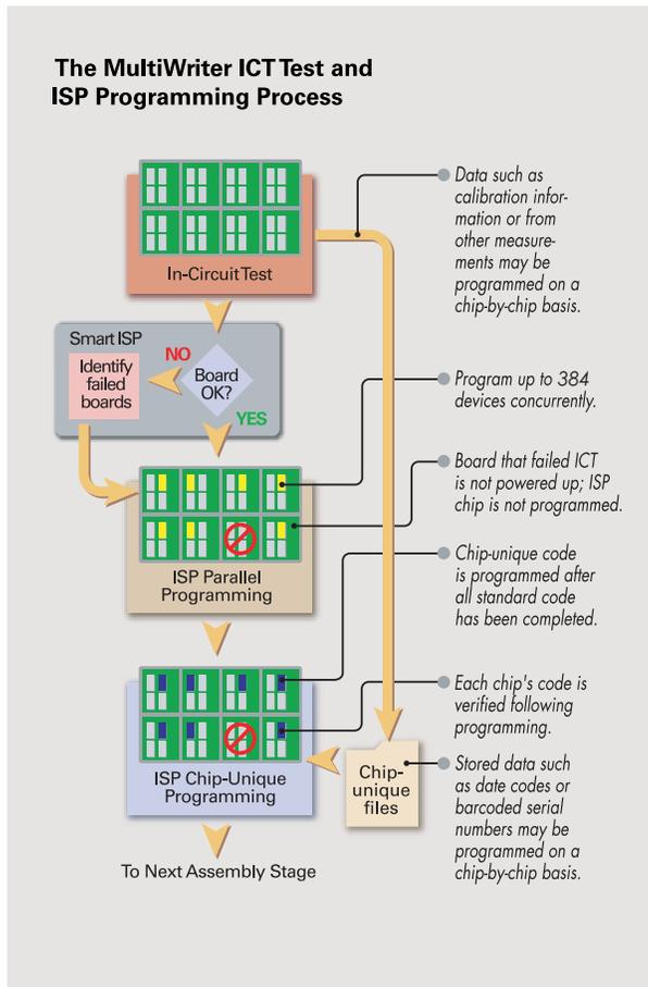
ISP programming follows a power-off in-circuit test. Smart ISP™ ensures that board power is applied only to those boards in a multi-board panel assembly that have passed the in-circuit test, ensuring that components are not inadvertently damaged. Standard code for all ISP parts is programmed simultaneously followed by chip-unique program code on a per-device basis.
